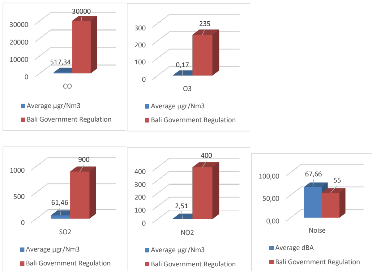
Figure 2: Average air chemical quality parameters CO, O 3 , SO 2 , NO 2 and noise levels in Denpasar City in 2021
