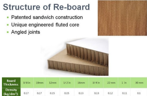
Figure 2. Re-board Structure (AimCulture Co., Ltd)
