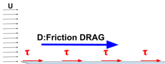
Figure 6: Expected friction drag and shear stress and their directions on a flat plate
